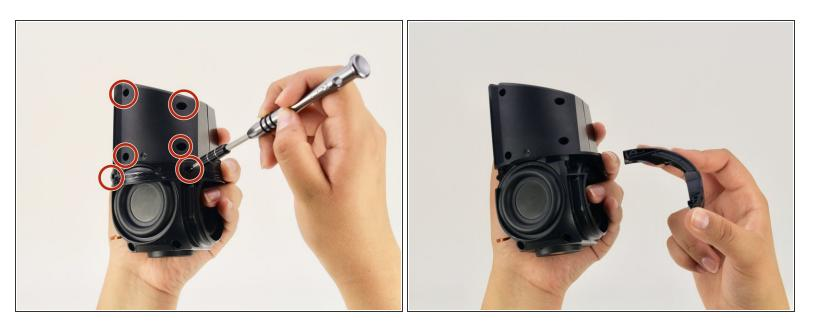
Using a Torx T6 screwdriver head, unscrew the six black 1.7mm Torx screws on the side of the device.
