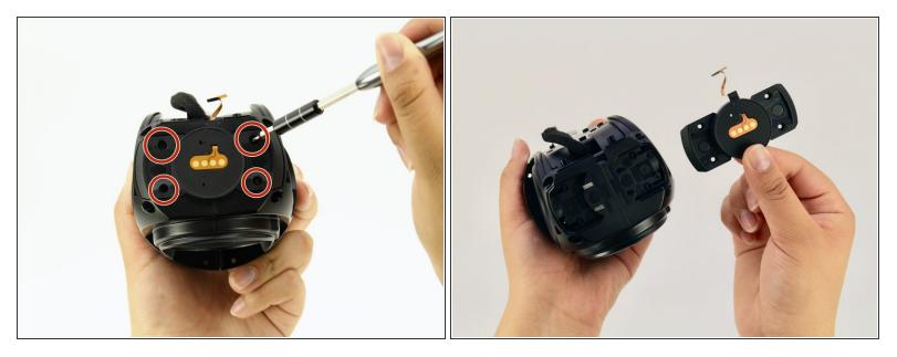
Using a Torx T6 screwdriver head, unscrew the four black 1.7mm Torx screws on the bottom of the device.
