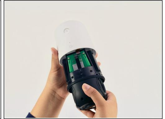
**⚠** Removing the lid too quickly could cause you to tear the interconnect cable that attaches the base to the top of the lid.
