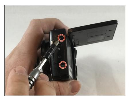
Remove the two 3 mm Phillips #000 screws on the side of camera with the flash toggle.
