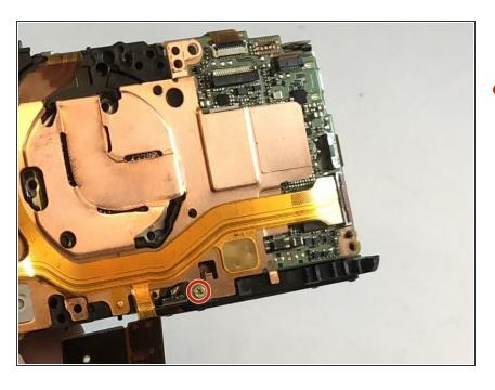
Remove the 5 mm Phillips #000 screw from the copper plate.
