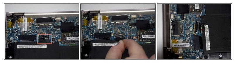
Using an iFixit opening tool and your other hand, gently lift the connector up from the tape wrapped around the connector wires and pry the connector from the motherboard.
