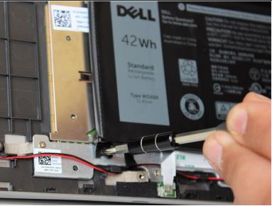
Remove the two 7.8 mm long screws on the left side of the battery with the Phillips #1 screwdriver.
