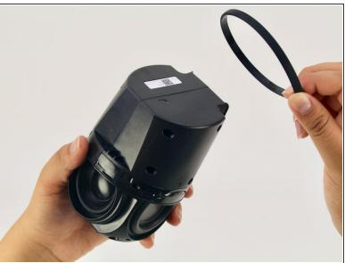
Remove the 'O-ring' that wraps around the device holding the switch panel in place.
