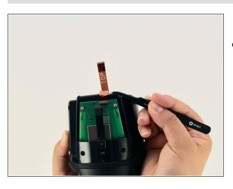
Carefully remove the interconnect cable using a pair of tweezers.
