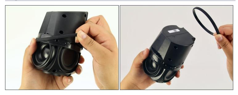
• Remove the 'O-ring' that wraps around the device holding the switch panel in place.
