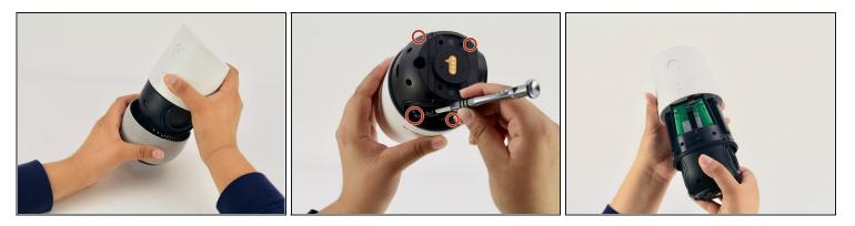
A Removing the lid too quickly could cause you to tear the interconnect cable that attaches the base to the top of the lid.
