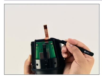
Carefully remove the interconnect cable using a pair of <u>tweezers</u>.
