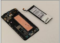
• With the motherboard removed, slowly pry off the battery with tweezers, starting at the bottom.
