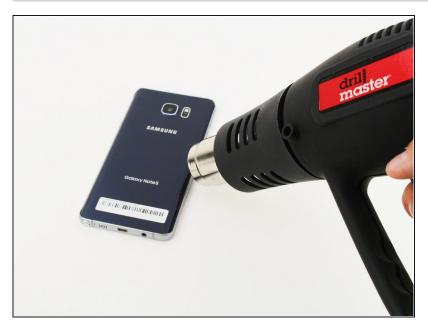
Heat the back of the device with a heat gun for two minutes.
