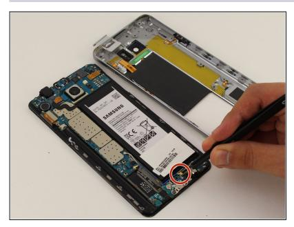
• Loosen the two signal cable connectors.
