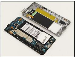
• Grip the back of the device and press down on the white square to remove the middle housing.
