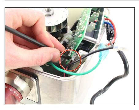
Pull or pry off the last connector block, then remove the control board.
