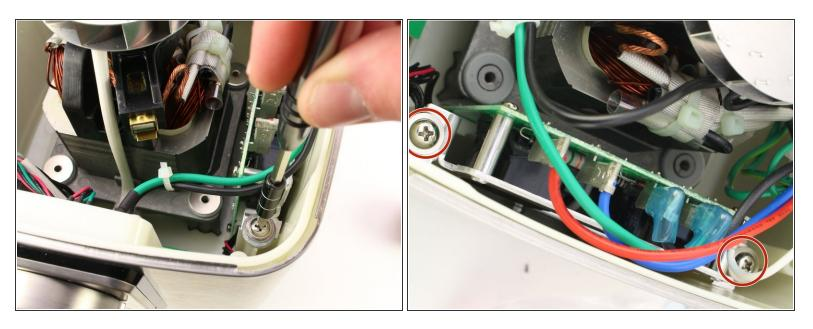
Using the same Phillips #2 screwdriver, remove the two 3/4" long screws holding the control board in place.
