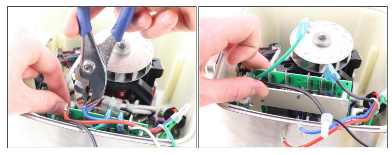
Using pliers, pull off all the connectors on the top.
