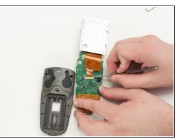
• Use tweezers to pull the two white pins on the connector forward.
