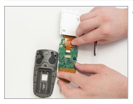
Remove the screen ribbon connector and screen.
