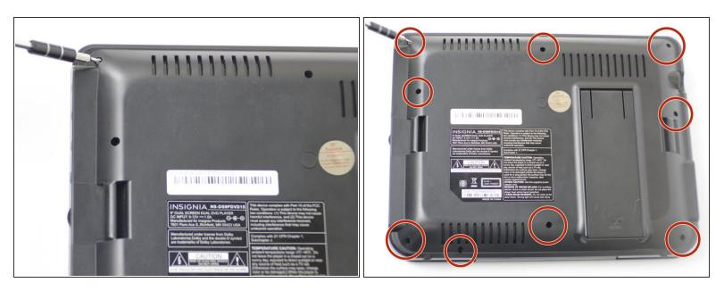
Unscrew the nine 9mm screws with a JIS #000 screwdriver.
