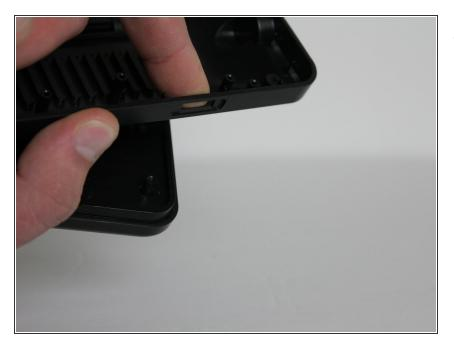
After the back is removed and you can see the interior of the device, push the old latch out.
