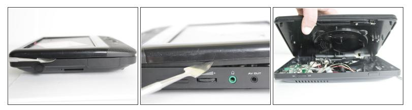
• Pry off back panel with prying tool, then remove by hand.
