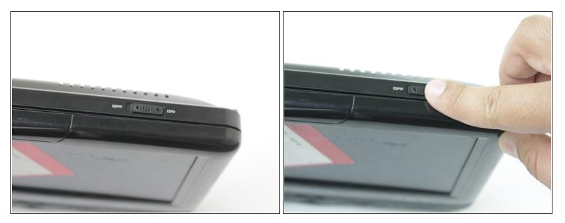
• Turn the power off. Slide the power button to OFF.
