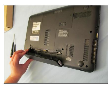
Remove the battery by pressing the two slider buttons in the appropriate direction.
