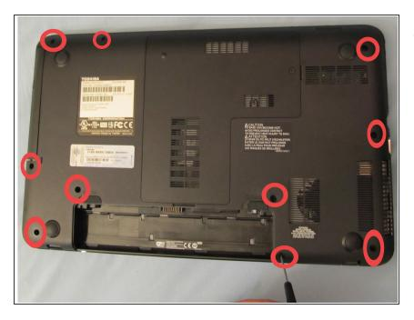
Next, remove the 10 screws located in the image. They are all on the bottom of the machine.
