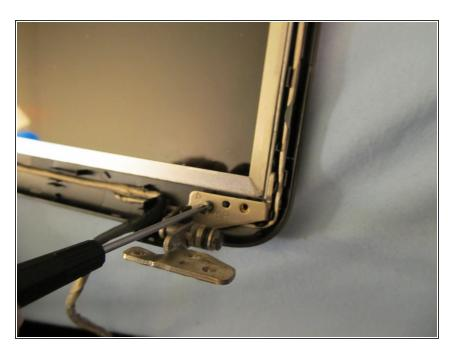
After the bezel is removed, unfasten two revealed screws: One on the right hinge, one on the left.
