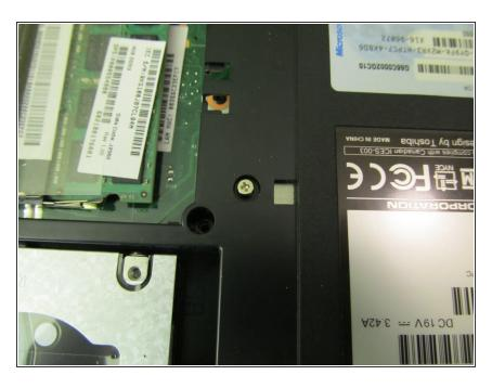
Next, remove the single screw holding in your DVD drive. After this screw is removed, your DVD drive will slide right out. Remove it.
