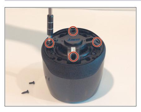
Remove the four 7mm Phillips screws from the plastic cover.
