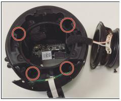
• Remove the four 7mm Phillips screws to expose the motherboard.
