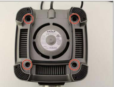
With the bottom of the blender facing up, use a Phillips #2 screwdriver to remove the 4, 1/2 inch long screws in the corners of the device.
