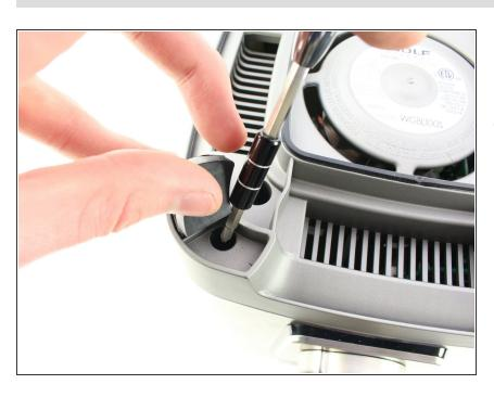
Using the same Phillips #2 screwdriver, unscrew the 1/2 inch long screw under each of the feet.
