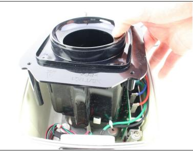
Pull off the base and remove the plastic housing underneath.
