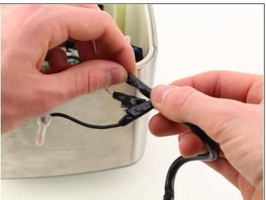
Wrap all the connections in electrical tape or heat shrink tubing.
