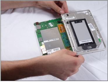
• Carefully lift the silver midframe away from the motherboard and display assembly.
