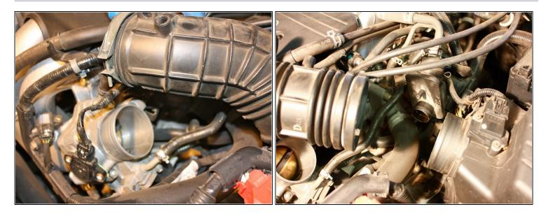
Once the screws are loose, completely remove the air duct hose by gently wiggling it off the engine and the air filter housing.
