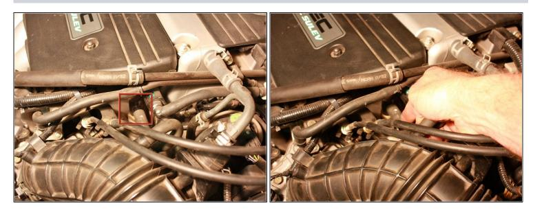
Remove the smog hose by squeezing the tubing and pulling it off.
