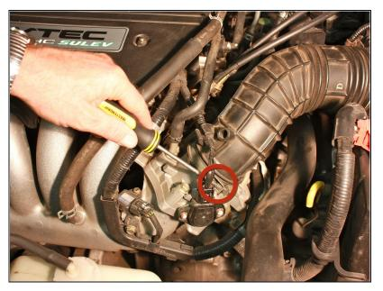
Using a Phillips screwdriver, loosen air duct clamp screws.
