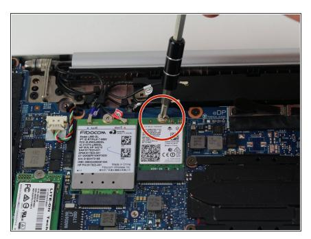
Remove the single 2mm screw that is holding the WiFi card in place using the Phillips #1 screwdriver.
