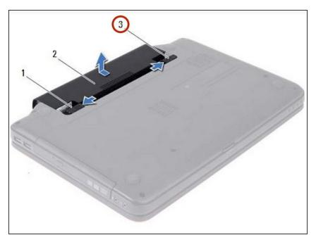
• Slide the battery lock latch to the unlock position until it clicks into place.
