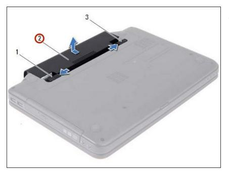
• Slide the **NEW** battery into the battery bay until it clicks into place.
