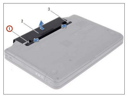
• Slide and hold the battery release latch in the unlock position.
