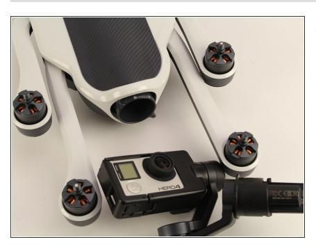
Remove the stabilizer by pulling the entire stabilizer out of the drone body.
