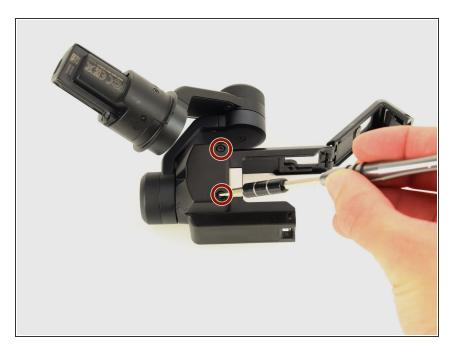
Using a Hex 2.0mm screwdriver, remove the two 12 mm hex screws closest to the harness.
