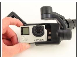
Place finger on the tab to open the harness and remove the camera.
