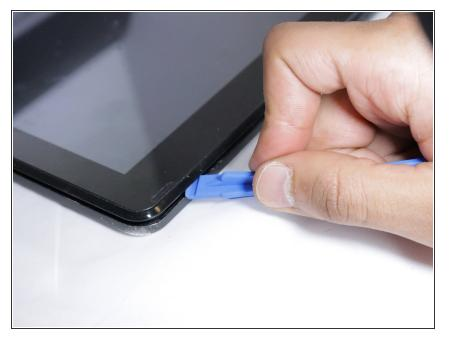
Use the plastic opening tool to pry the front edges of the screen off of the back.
