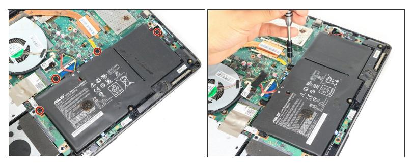
• Unscrew the four screws to remove the battery.
