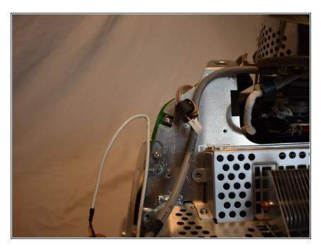
The power button cable may be tucked in the casing, you will need to un-tuck it.
