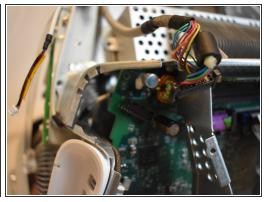
There is a large display connector that must be removed. This can be done by squeezing the tabs and pulling.
