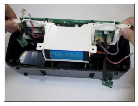
Slightly lift the white box with all the wires still attached.
