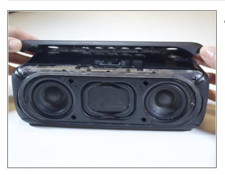
To save time, pry up and remove the top panel first.
