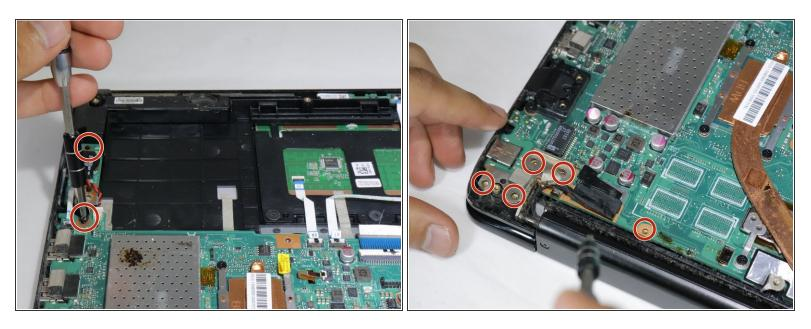
Unscrew the seven screws Phillips Head 0.0793 MM on the edges of the motherboard.
