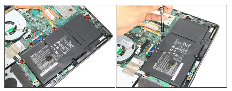
Unscrew the four screws to remove the battery.
