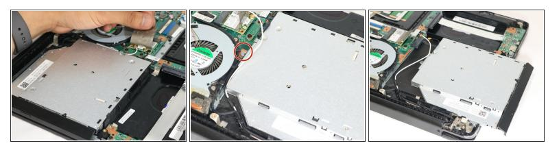
Lift up the sticker that sticks between the motherboard and the optical drive. Then, unscrew the one screw where it is marked and slide it out gently.
