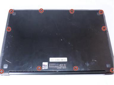
Unscrew the 10 screws around the edge of the back panel. Eight of the screws are 0.0793mm T5, two of them are 0.0793 JIS #0.
