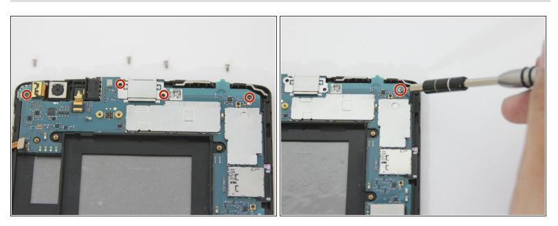
• With the Phillips #000 screwdriver, unscrew the four 4.0 mm screw that are holding down the motherboard.
