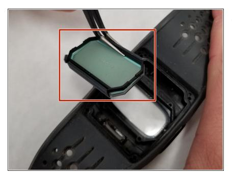
Remove the screen using tweezers.
