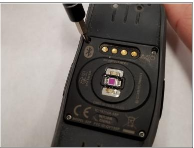
Remove the four 6.7mm JIS #00 screws from the back cover.
