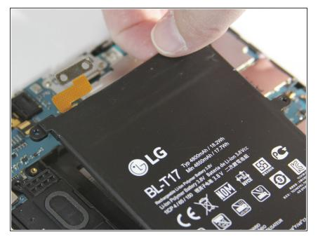
• Lift the battery with your fingers and remove it from the device.
