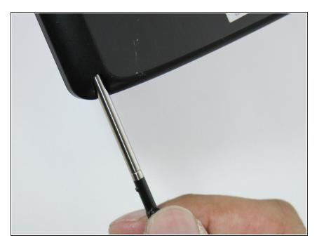
• Slide the stylus out from the bottom left corner of the back panel.
