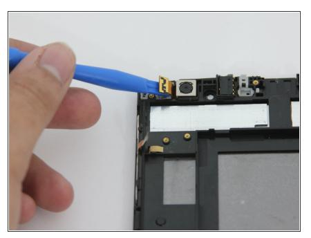
Insert the plastic opening tool under the ribbon connector that is holding the rear-facing camera down and lift it up.
