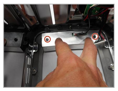
Remove two 8mm screws securing the lighting component using a Tripoint Y1 screwdriver.
