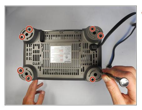
Remove the eight 8mm screws on each toaster foot using a Tri-point Y1 screwdriver.
