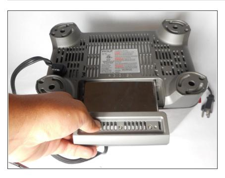
Remove the crumb collector located on the bottom of the toaster.
