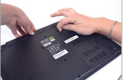
Slide the locking latch to the right and hold while pulling the battery out with your other hand.
