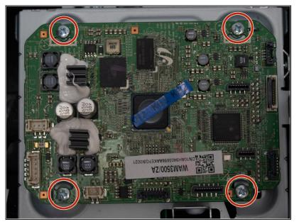
• Remove the four 12mm long screws with the Phillips #1 screwdriver.
