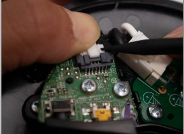
• Remove the connector from the board by pressing down on the center tab while nudging the connector away with a spudger.
