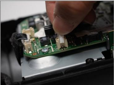
• Disconnect the six plugs on the motherboard.
