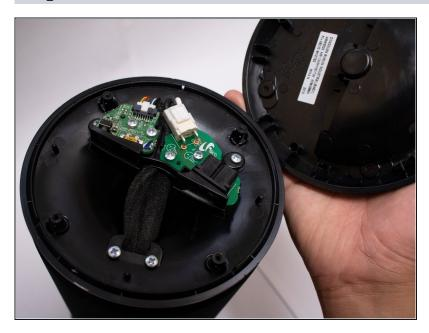
• Remove the bottom shell from the speaker.
