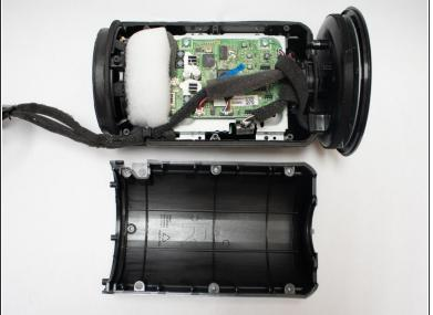
Pry the two halves of the body open using a metal spudger.
