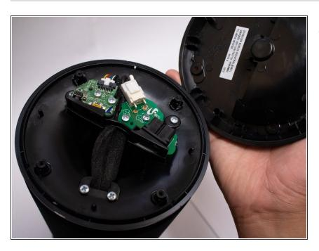
Remove the bottom shell from the speaker.
