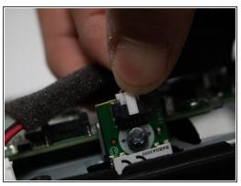
Remove the plugs located topmost right and closest to the bottom in picture.
