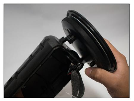
• Remove the touch panel by sliding it off the end.
