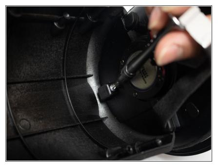
• Remove the six 12mm screws with the Phillips #1 screwdriver.
