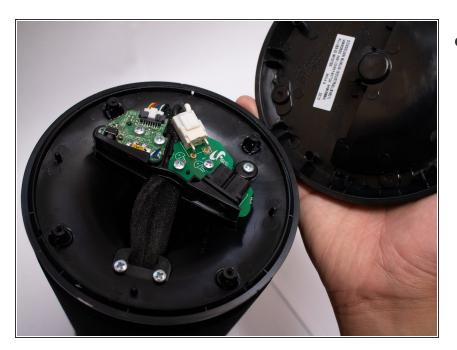
Remove the bottom shell from the speaker.
