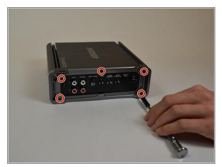
Remove the five T10 Torx screws from the housing.
