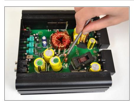
Desolder the capacitor and remove.
