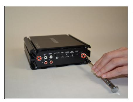
Remove the two T10 Torx screws from the faceplate.
