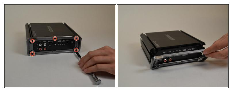
• Remove the five T10 Torx screws from the silver face plate.
