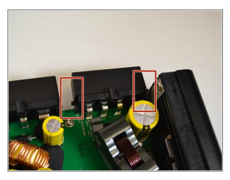
Pull apart black tabs on plastic housing for output connections.
