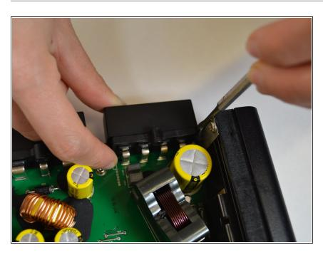
Desolder the four audio jack connectors from the motherboard.
