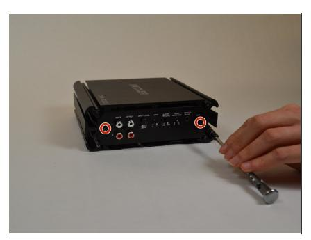
Remove the two T10 Torx screws.
