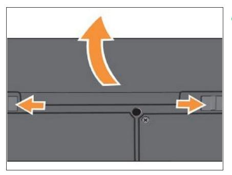
Slide the battery lock switch to the right into the unlocked position.
