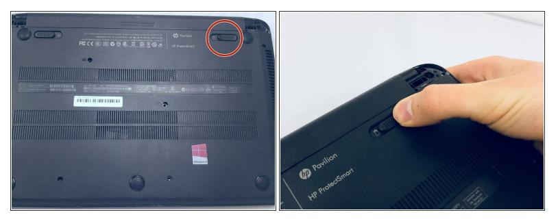
Press the switch on the right-hand side of the back of the device towards the center until the gray battery icon is no longer visible. This will eject the battery.
