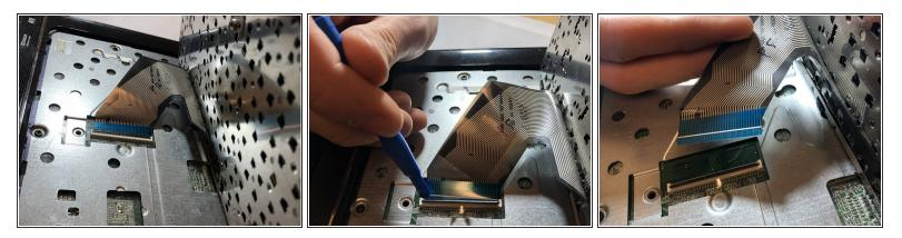
• Push the button to release the connector and pull it out and remove the keyboard
