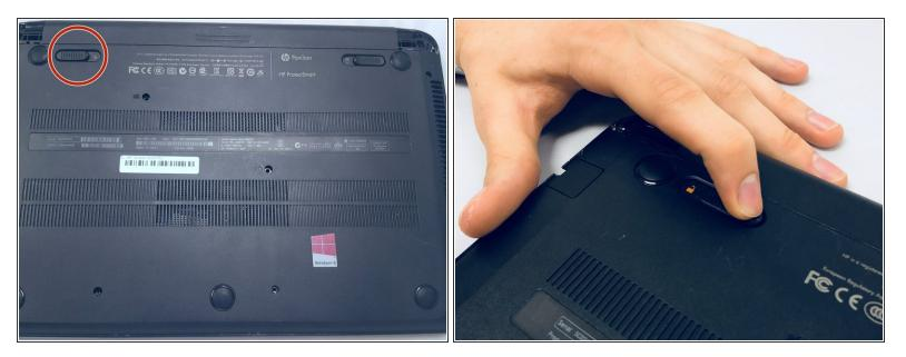
Flip the computer over and move the battery lock switch to the "unlocked" position (marked by an orange lock icon).
