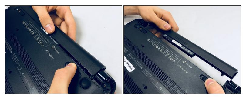
• Carefully pull the battery away from the device.
