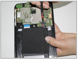
• Using the spudger, gently press on the black button on the plug port to release the battery from the plug.
