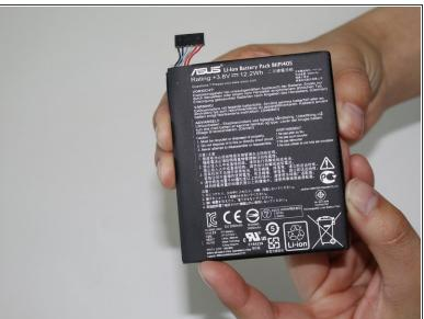
Remove the battery from the device.
