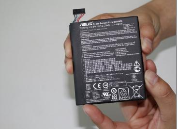
• Remove the battery from the device.
