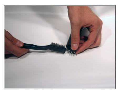
Using a detailing brush, gently brush the pins and inside walls of the microphone.
