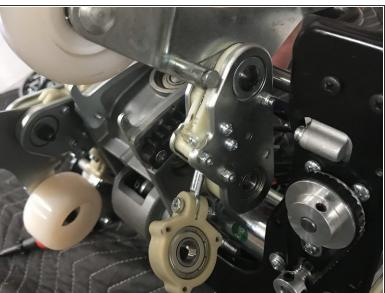
Using the handle of a wrench or a small pry bar apply pressure between the roller arm and the assembly.
