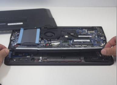
Carefully, lift up the battery-pack to remove it.
