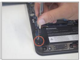
• Remove the 3 screws using the Phillips screwdriver #000. The screws are wafer-heads, size m2x4mm.
