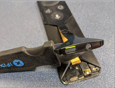
• From here you will want to use the Jimmy or similar item to get under the bottom corner to get past the inner clips. From here you can carefully get both sides of the bottom top cover and lift it off. The remainder of the cover should come off fairly easily. If not use the jimmy to unclip the others.
