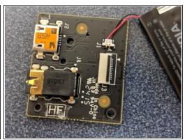
From here you can remove the Single Phillips Screw using the Phillips 00 Driver Bit. This will let
