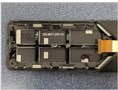
Once you have the Circuit out of the glue you will see the shown Ribbon attachment clip moved up to be removed. Second picture the board is removed.
