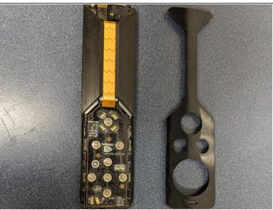
The Buttons are easily removed. The Volume Touch pad is also seen here; it is attached by glue.
