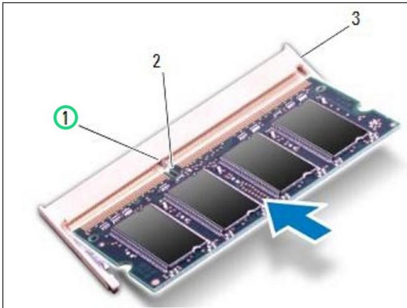
**!** CAUTION: If the memory module cover is difficult to close, remove the module and reinstall it. Forcing the cover to close may damage your computer.
