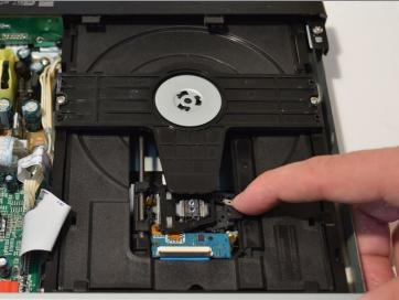
• To access the optical lens, pull back the optical drive as shown in the pictures located on the two metal rails.
