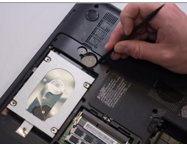
Push the pin that holds the CMOS battery in place downwards. The battery will then come out.
