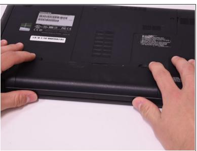
Use two fingers to pull the ridged lock tabs on the bottom of the computer toward the edges. This
