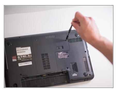
Remove the 7mm screw from the back panel using the Phillips head screwdriver.
