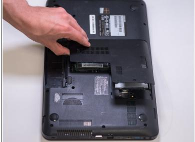
Use the spudger to pry the back panel out of the laptop.
