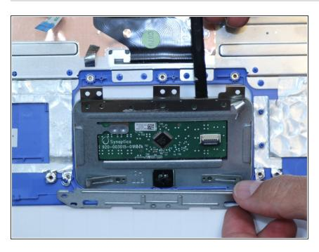
Use a plastic spudger to lift the trackpad away from the keyboard.
