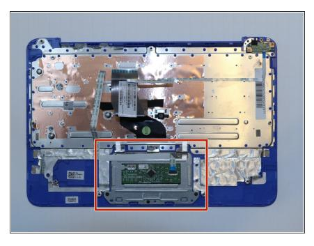
Flip the keyboard over to locate the trackpad.
