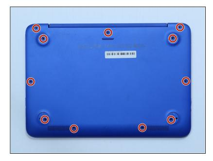
• Remove the eleven 5 millimeter housing screws from the bottom of the computer using a #00 Phillips head screwdriver.
