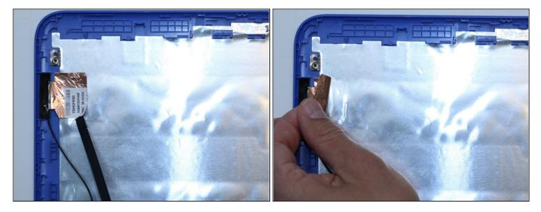
• Use a plastic spudger to peel away the copper filament.
